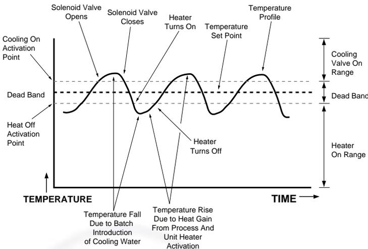
In the solenoid valve system, ALL of these factors, acting simultaneously, influence temperature stabilization:
