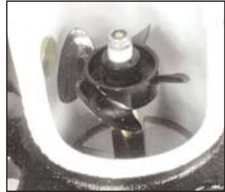
Cut away view of flow meter from the Sentra SK.
