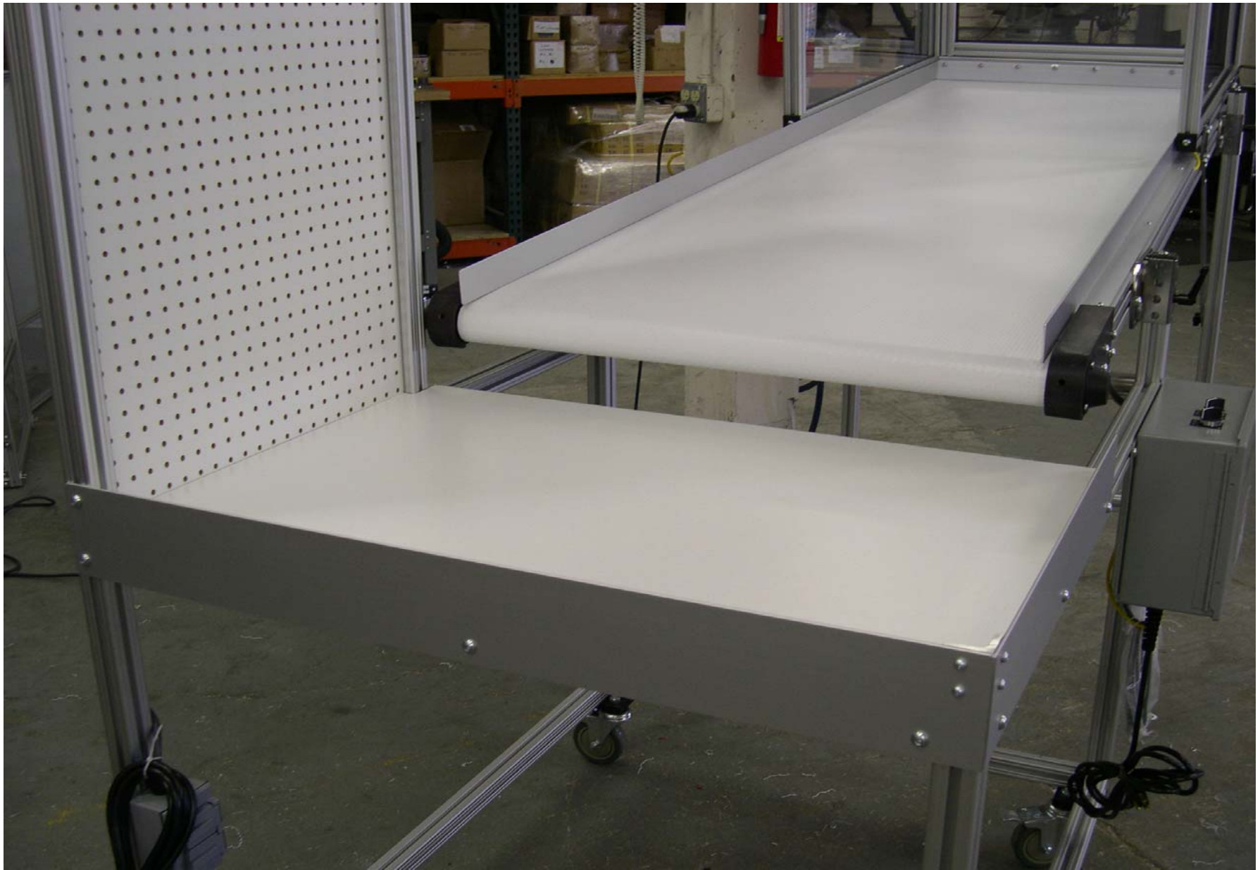
Work Table fed by HFA 2210 Series Conveyor
