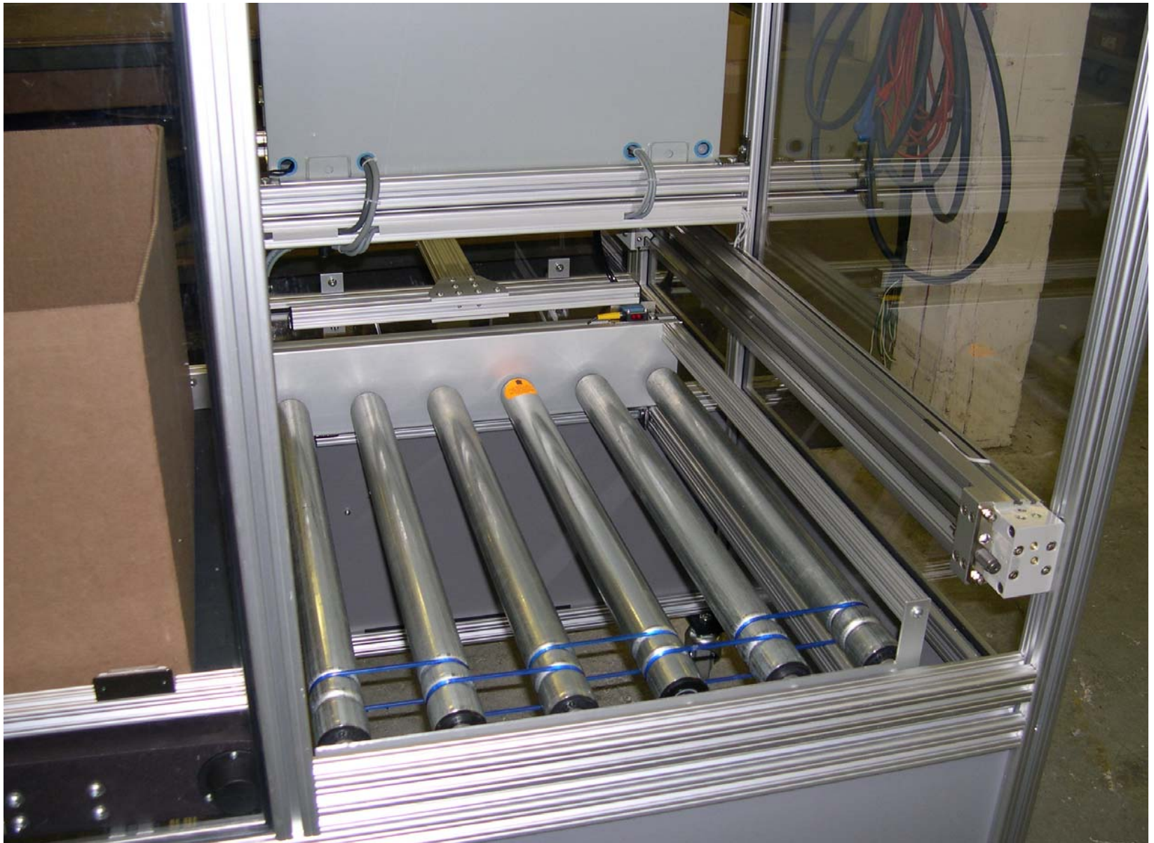
Weigh Scale Built into Box-Filling System
