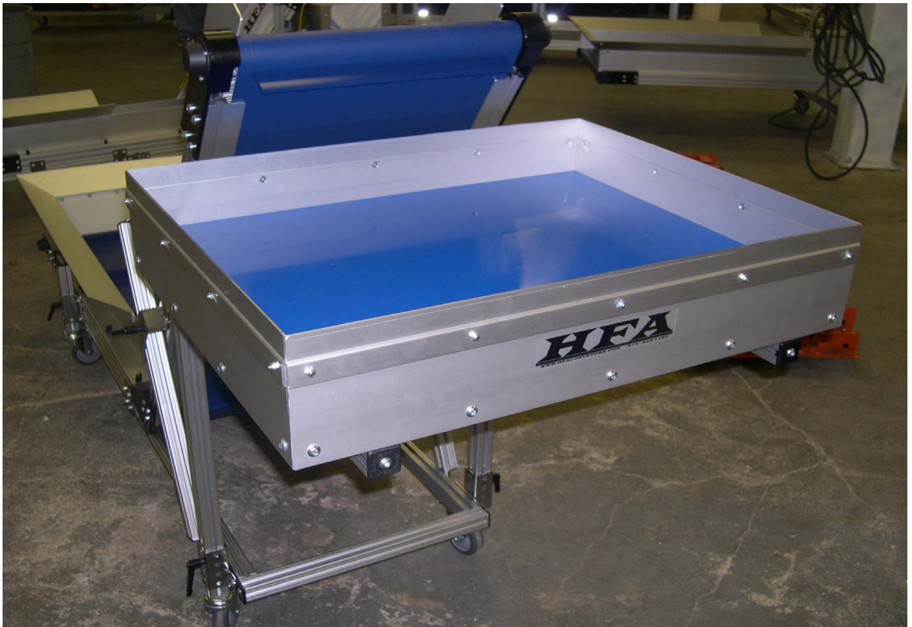
Work Station Mounted to an HFA 2230 Series Conveyor with Blue UHMW Surface
