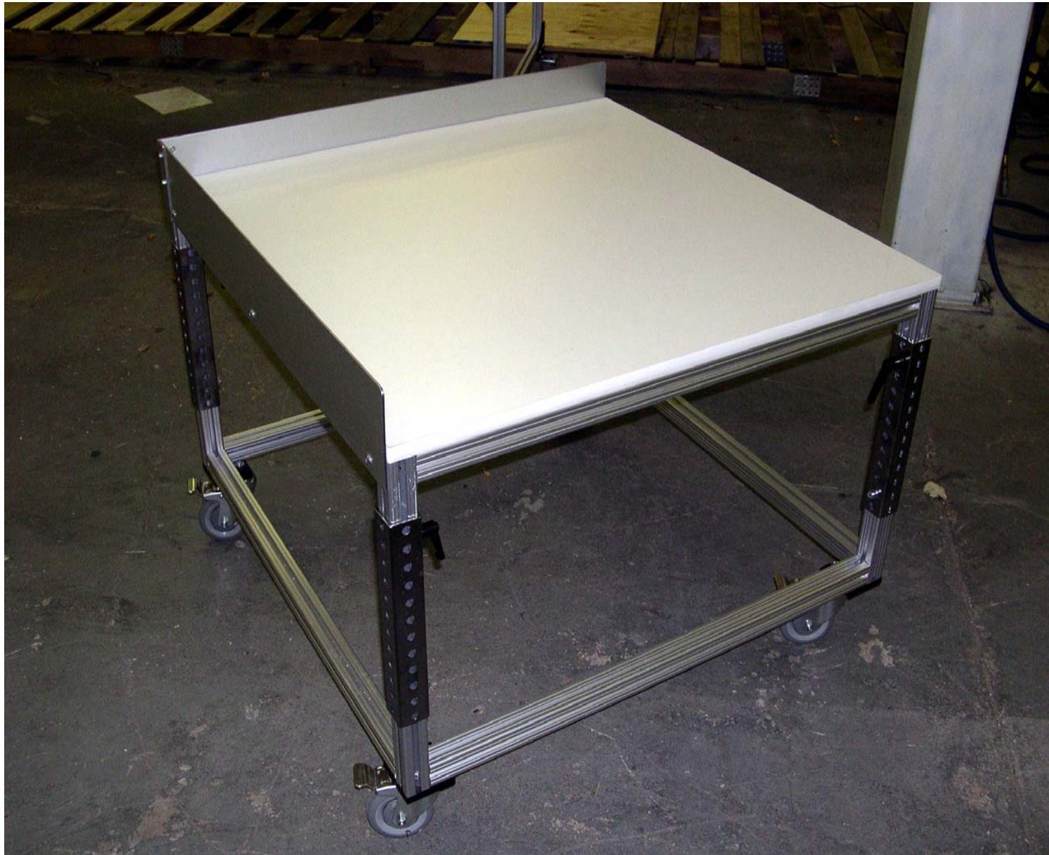
Work Station with Telescoping Legs and White Laminate Table Surface
