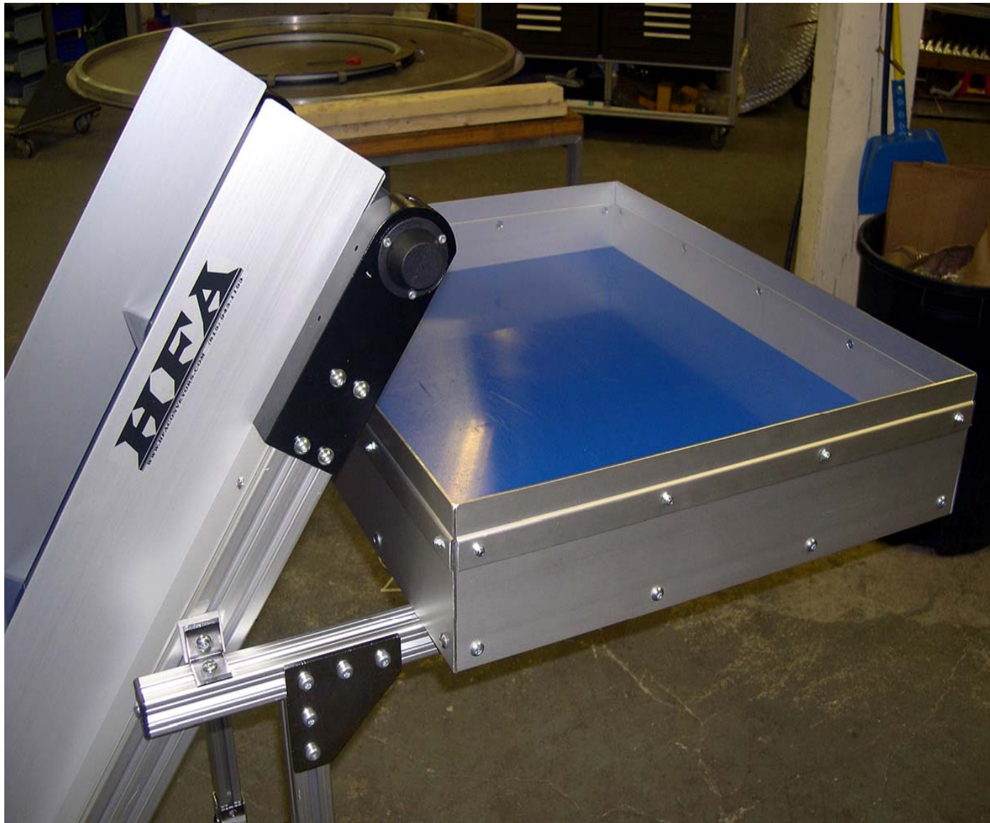
Work Station Mounted to Frame of Conveyor at the Discharge End
