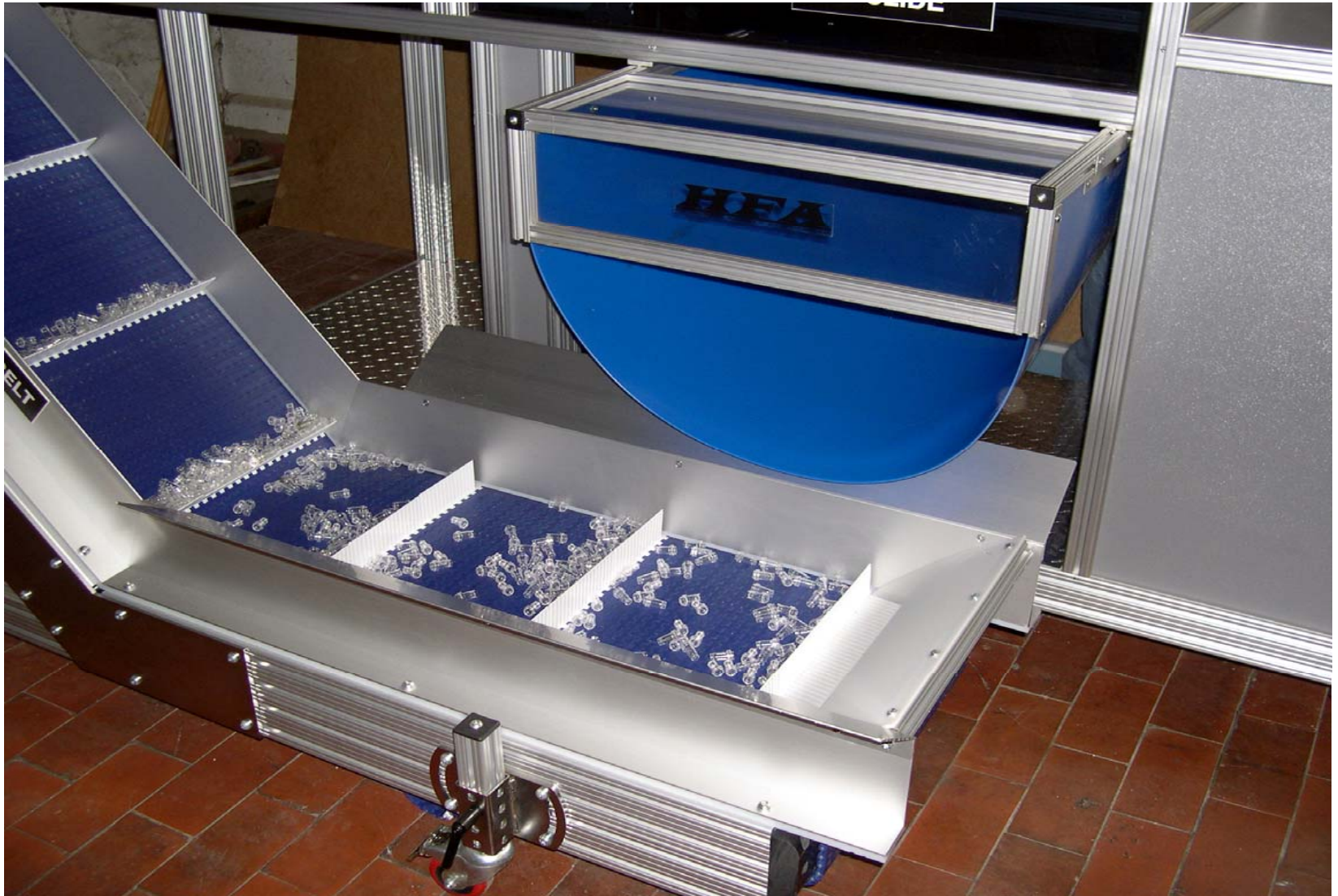
Under Press Chute Feeding an Aisle Conveyor
