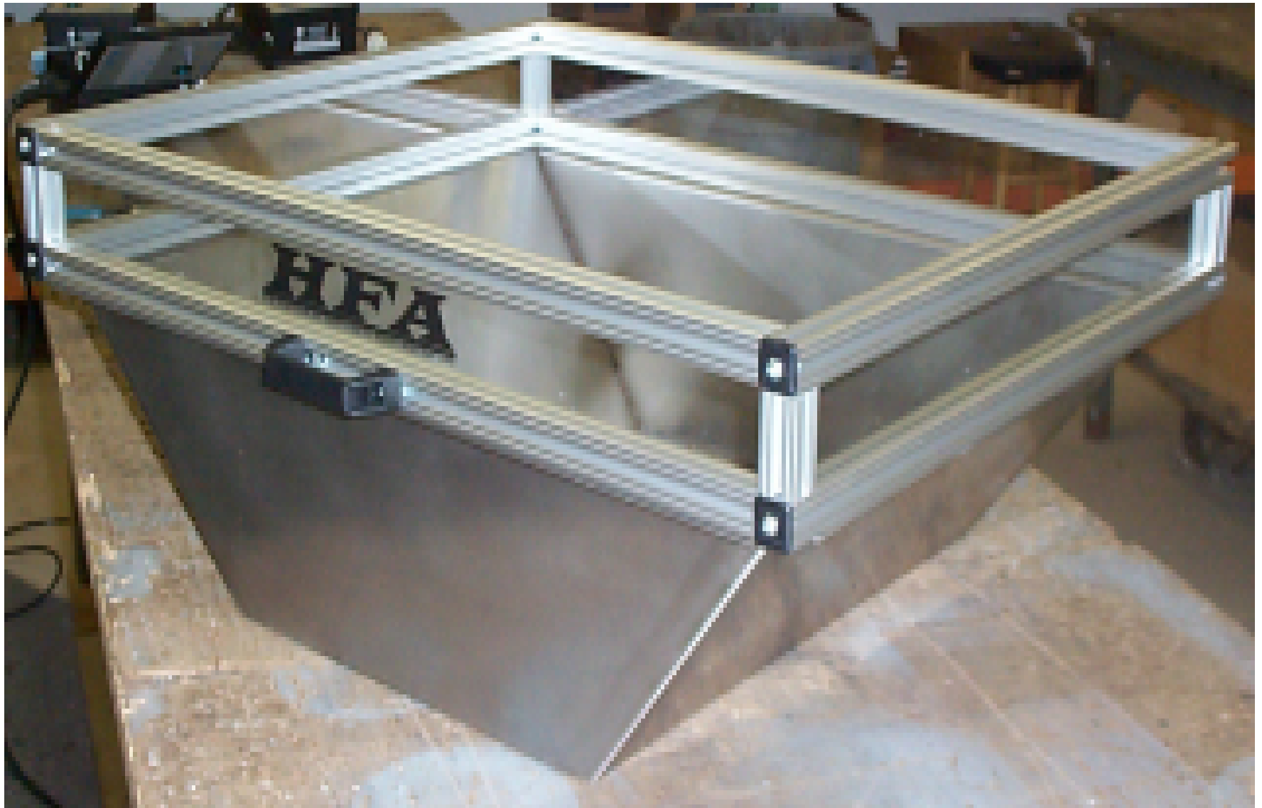
Stainless Steel Under Press Funnel Designed to Direct Parts Straight Down into Box or Under Press Conveyor
