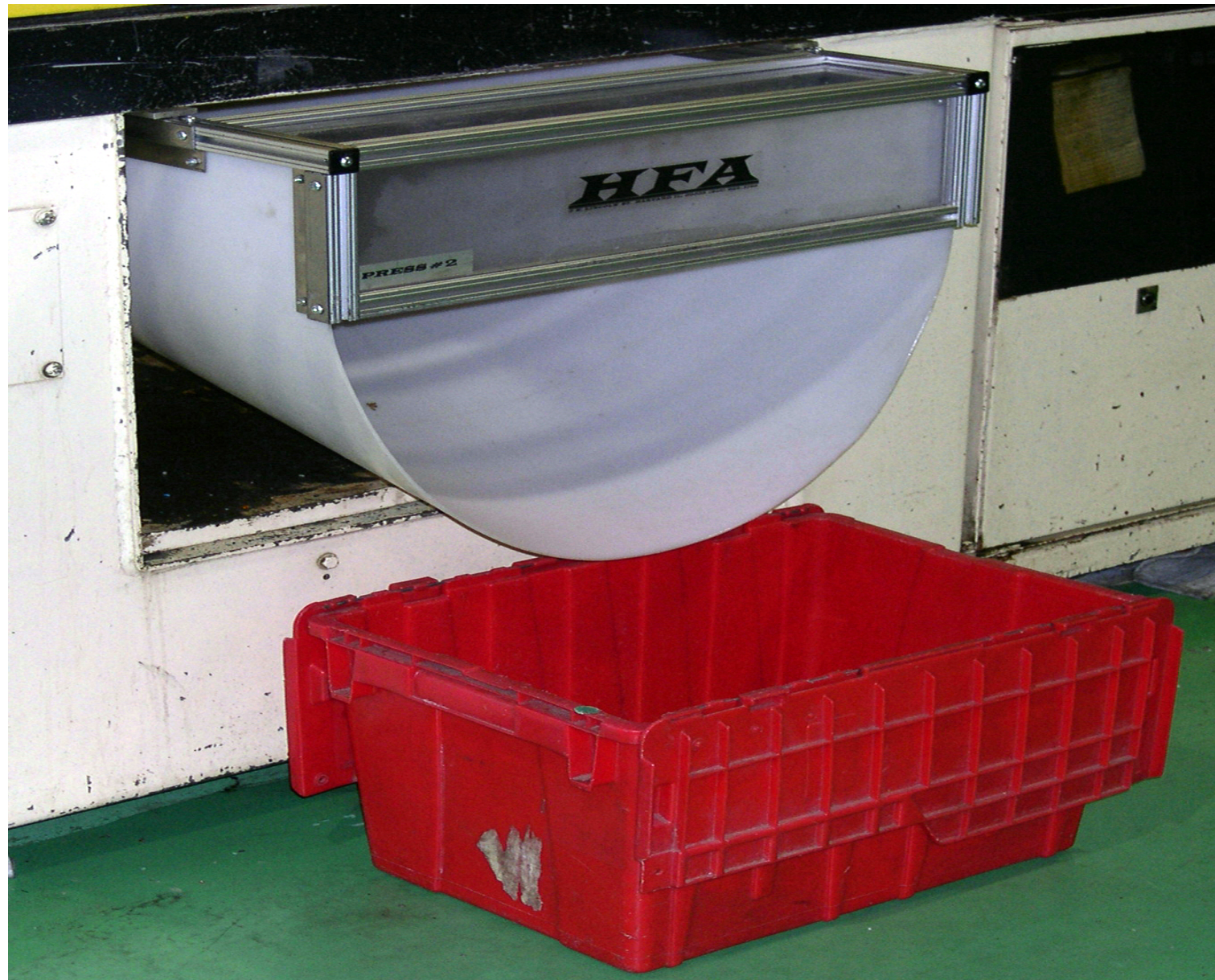
White UHMW Under Press Chute Feeding a Tote
