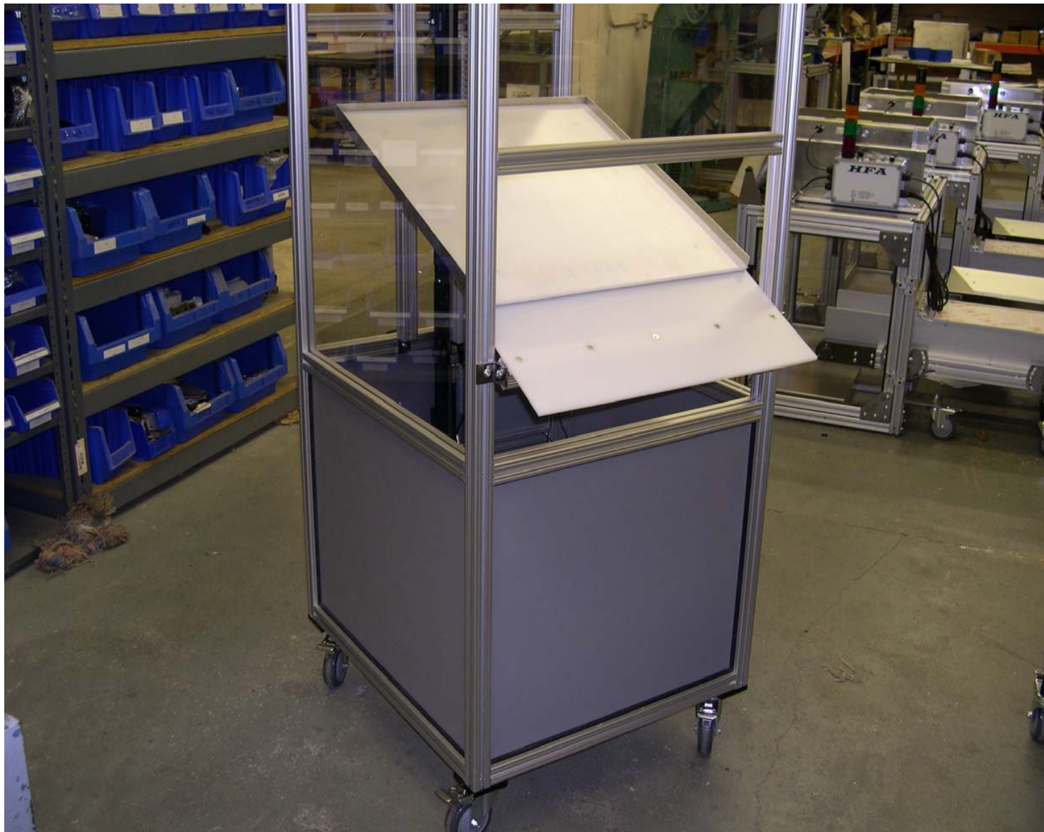
V-Lift with Discharge Tray and Lexan Guarding
