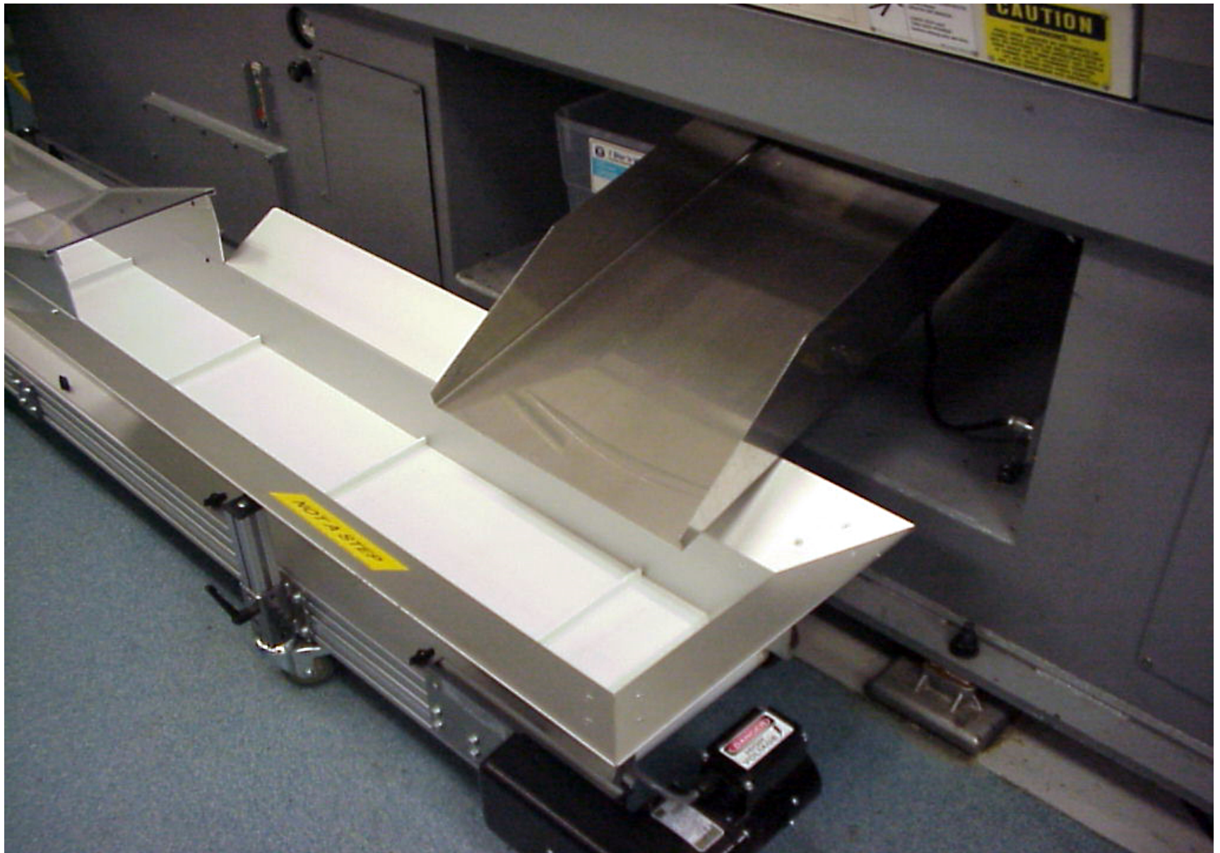
Stainless Chute Feeding an HFA 2230 Model Conveyor Outside Press
