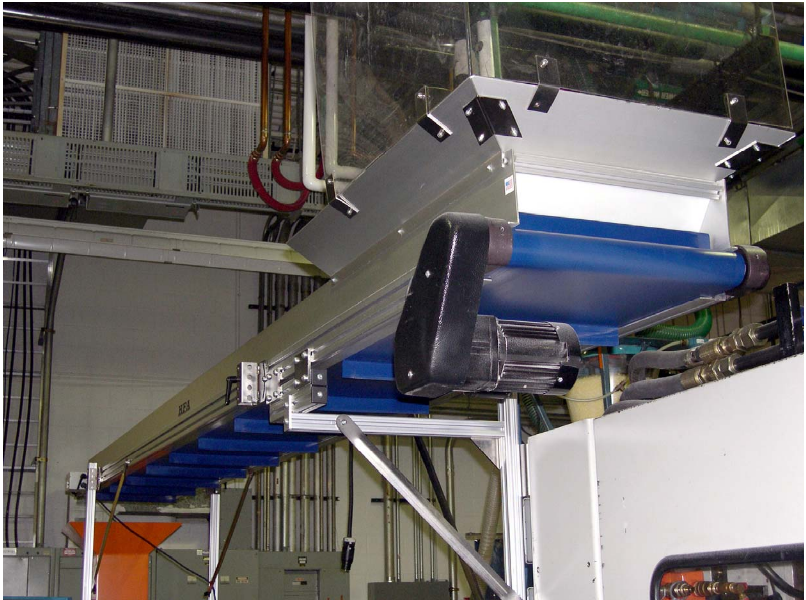
HFA 2210 Model Runner Conveyor Mounted Overhead
