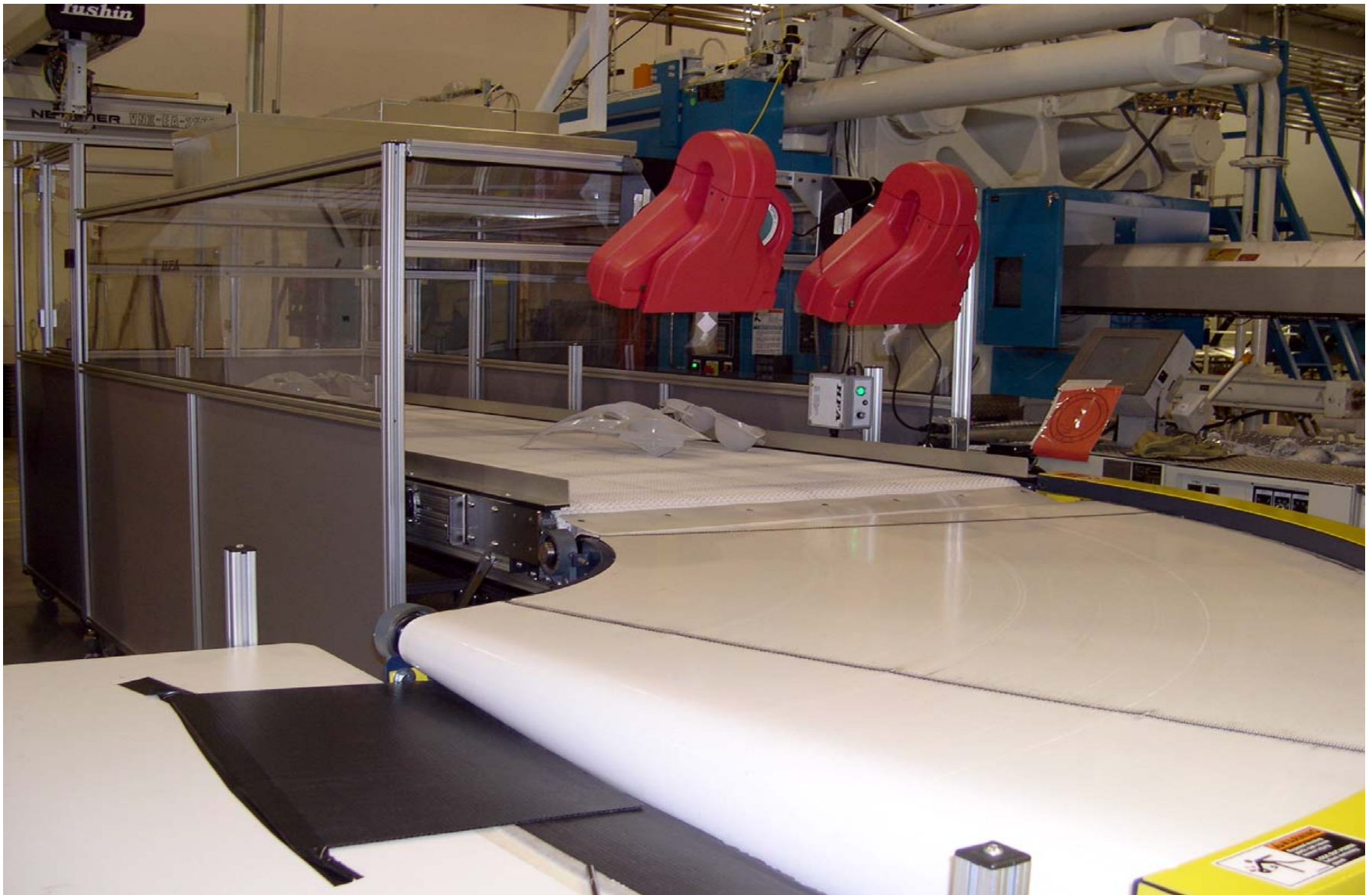
Static-Eliminator with an HFA Curve-Belt Conveyor
