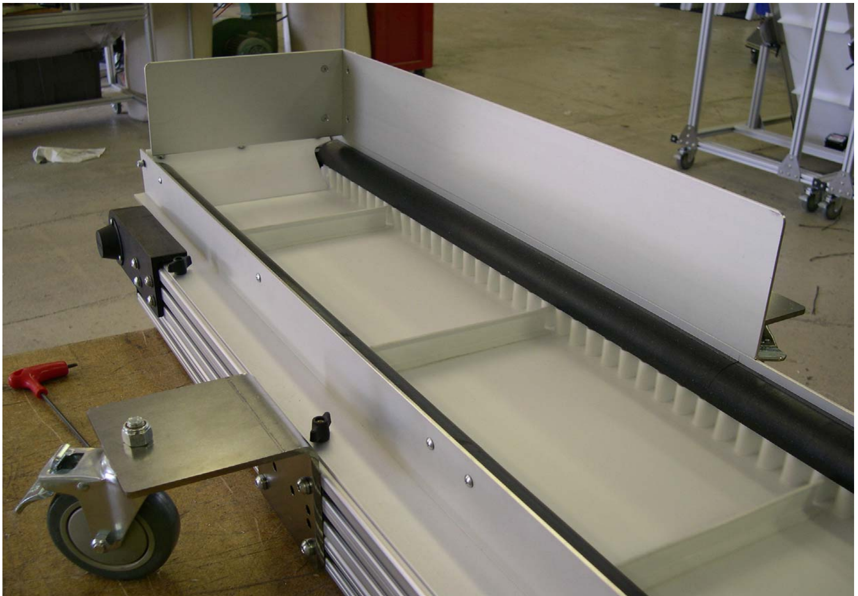
HFA 2230 Model Conveyor with Extended Rails at In-Feed, Outrigger Caster Plates and Corrugated Side Walls on Belt
