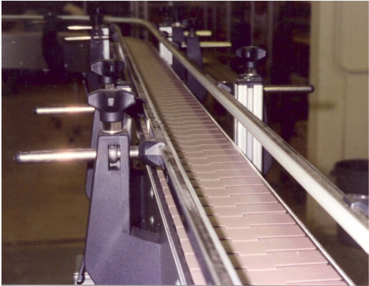
Plastic “Flexible-Style” Belt Conveyor with Adjustable Rail Guides for Different Size Parts or Containers
