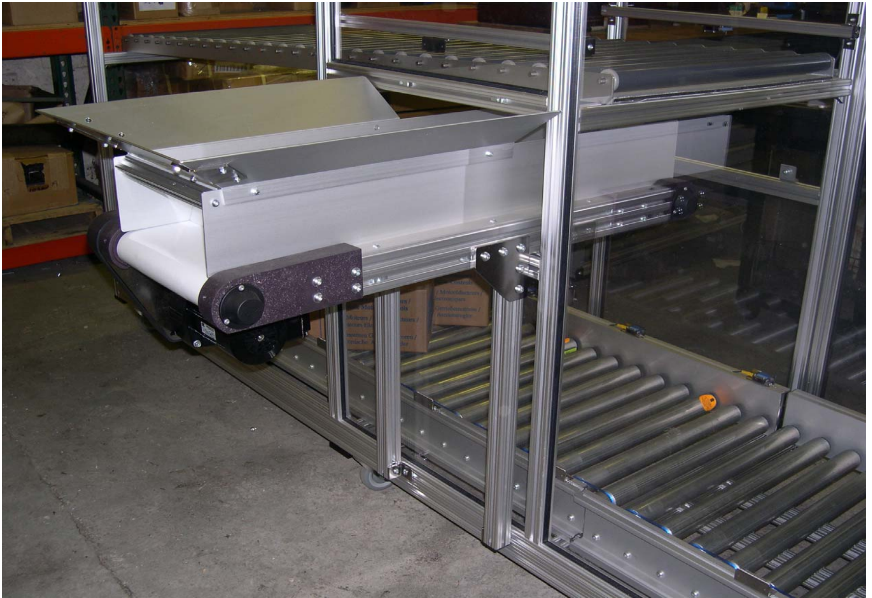
HFA 2210 Model Conveyor Mounted to Frame of HFA Box-Filling System
