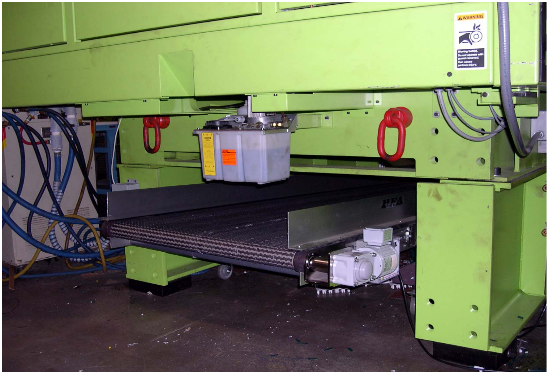
HFA Under Press Conveyor with Plastic Link Belting
