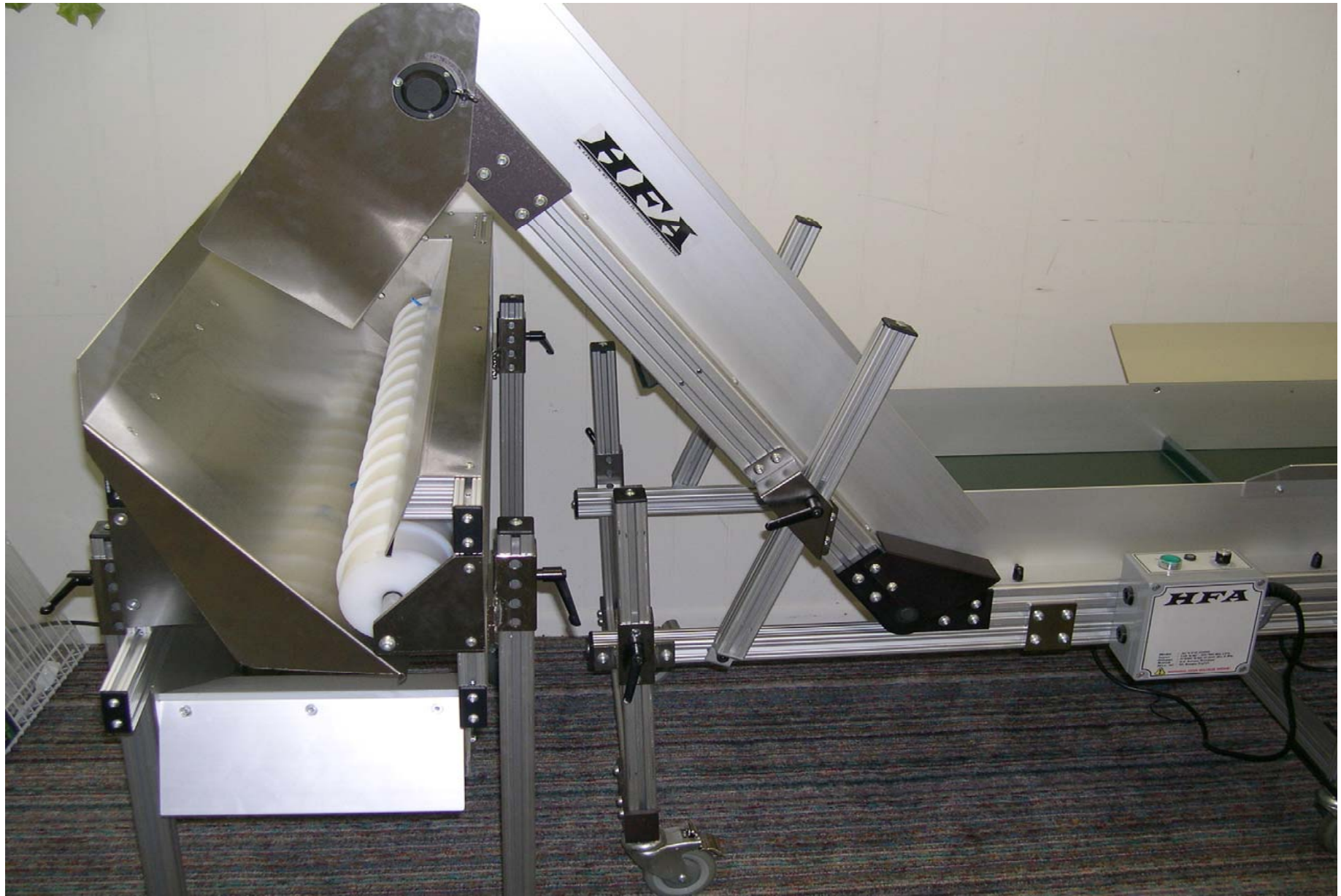
Auger Style Separator with White UHMW Screw Fed by Under-Press HFA 2230 Model Conveyor
