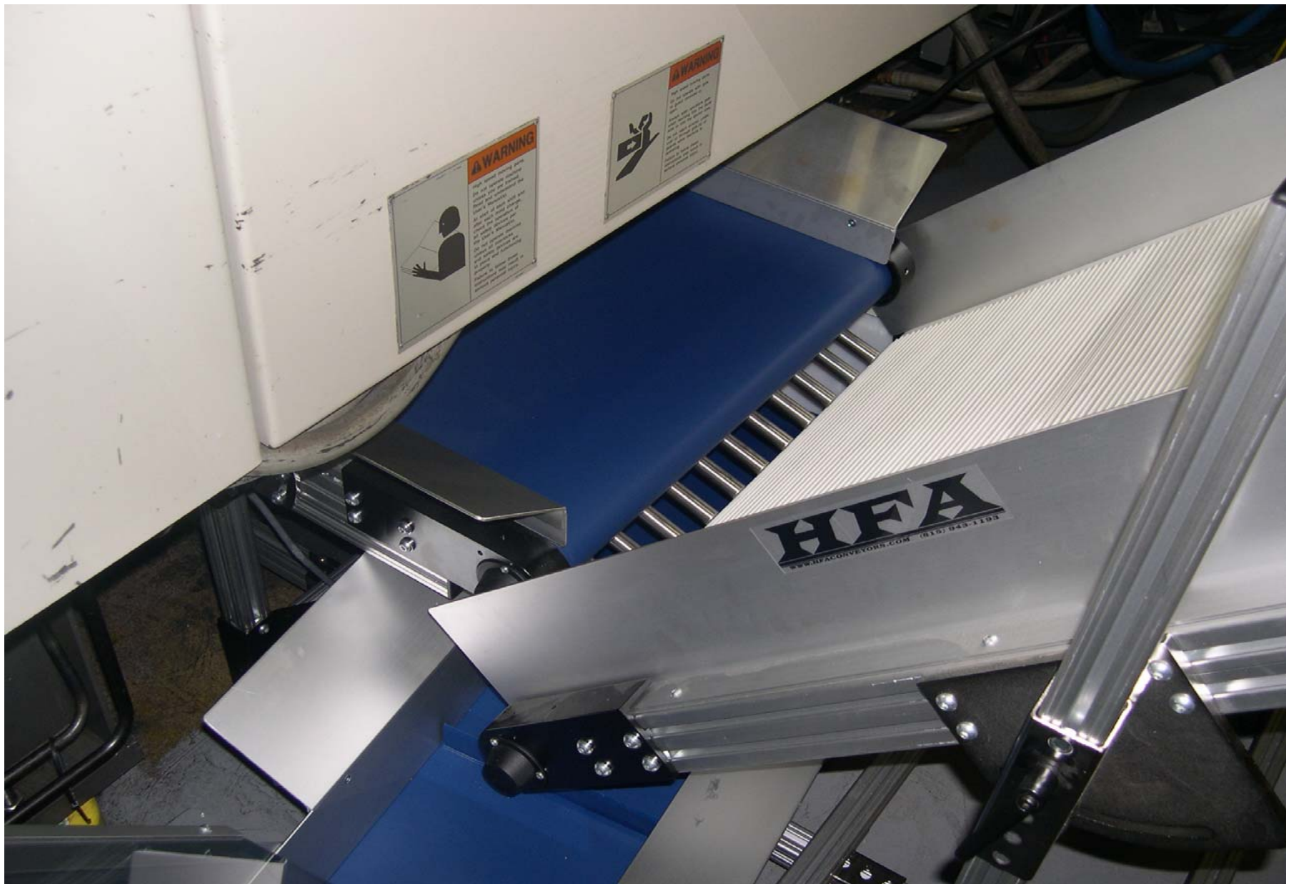
Stainless-Steel Bar-Type Separator with Textured Belt Separator Attached to an HFA 2210 Style Under Press Conveyor
