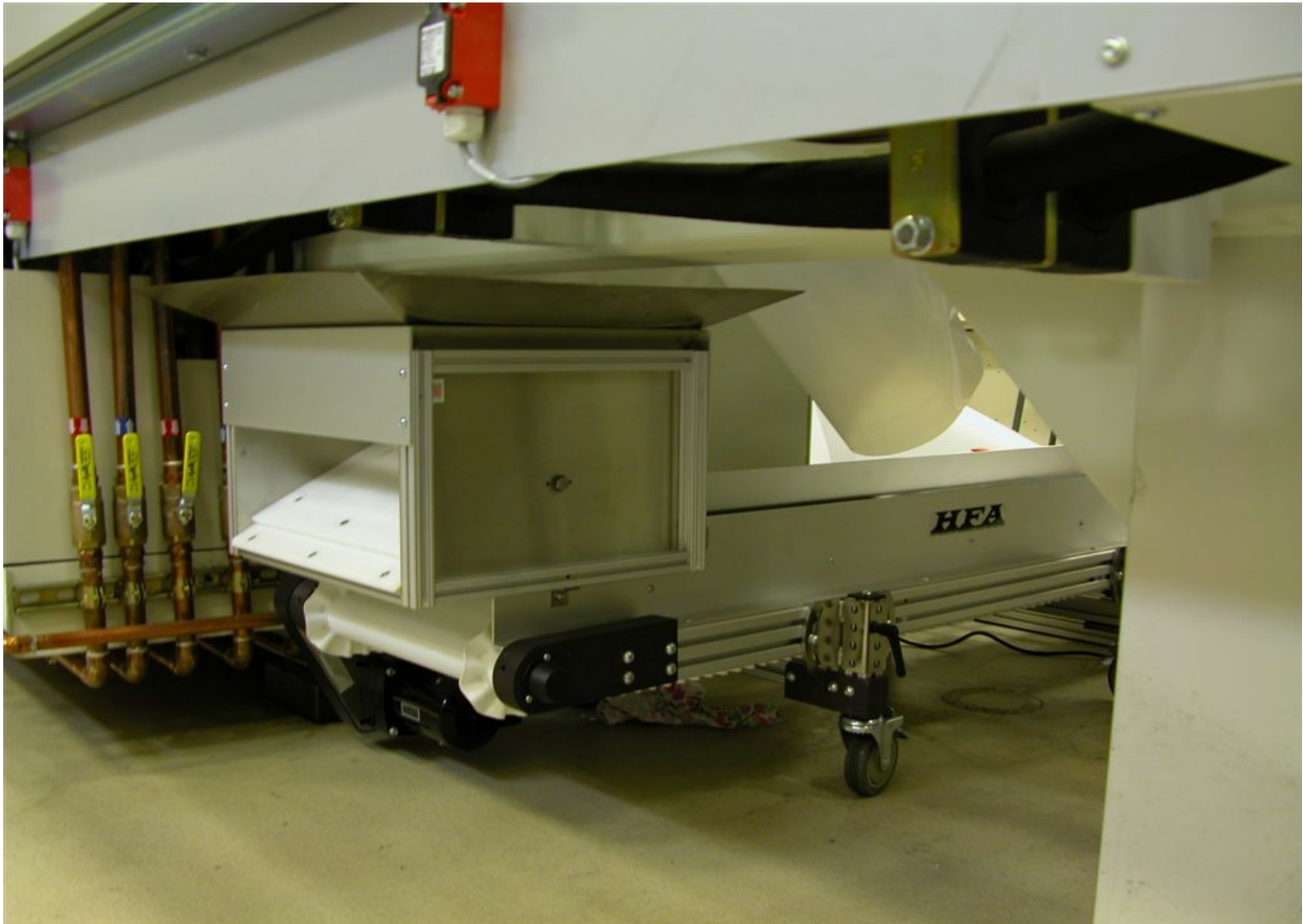
Diverter Mounted to Under Press Conveyor
