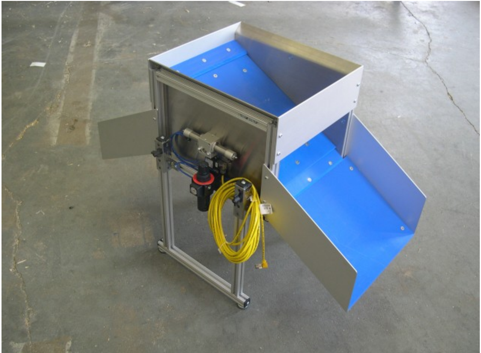
Under Press Diverter Shown with Rotary Actuator and Signal Cord for Press
