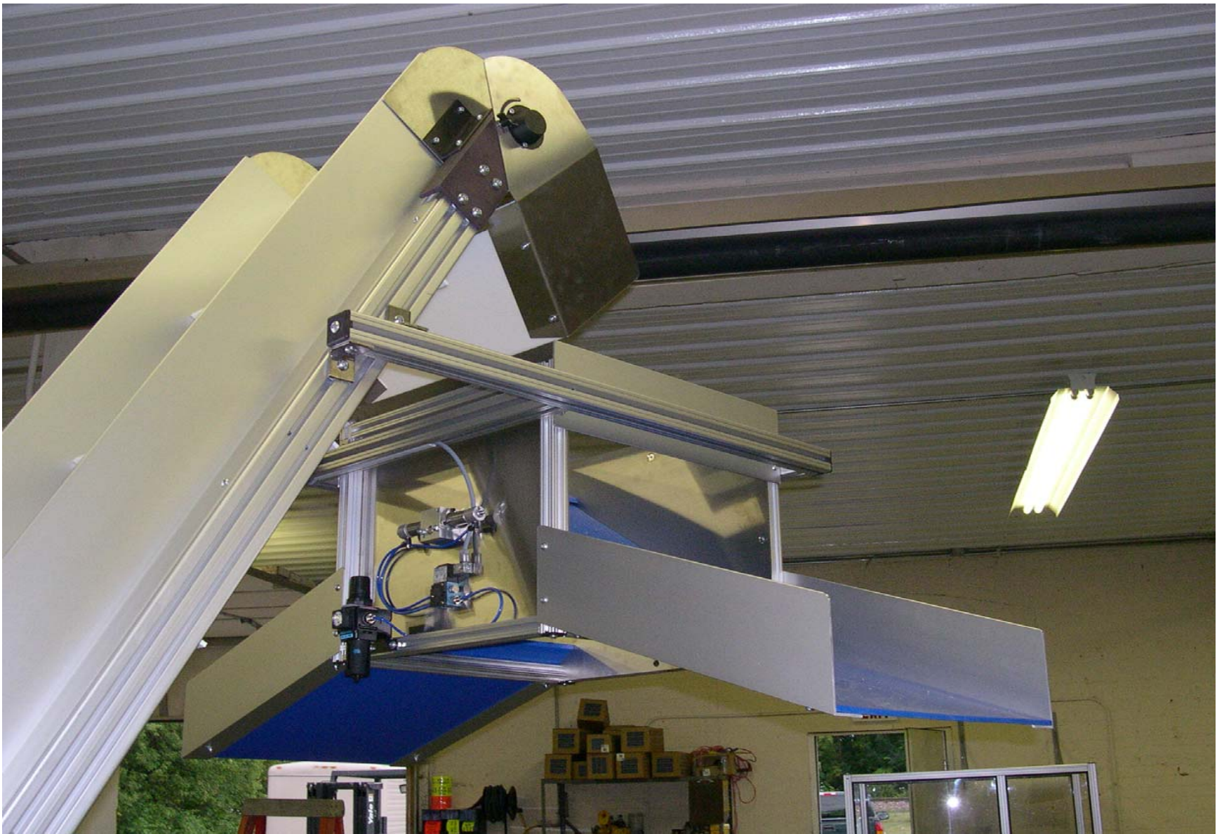
Diverter Mounted at Discharge End Showing Actuator
