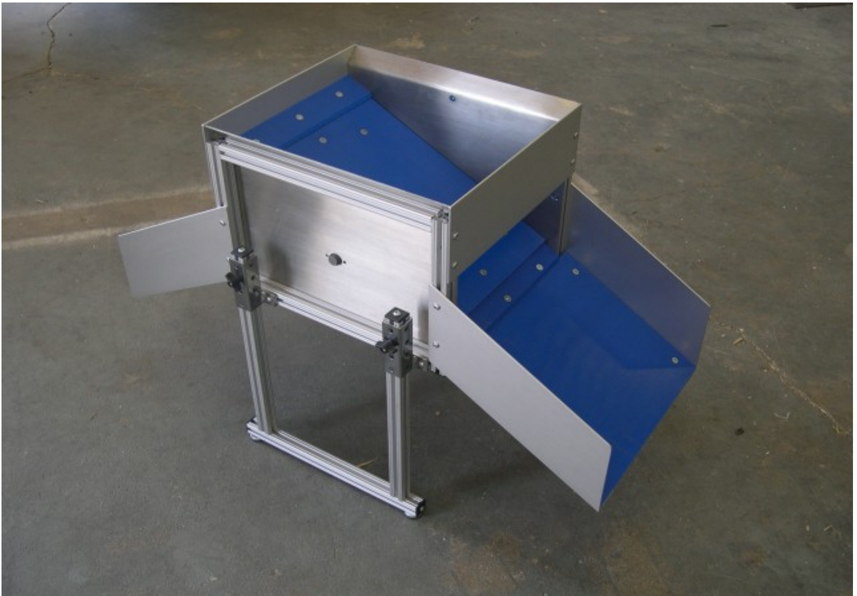
Under Press Diverter made with Blue UHMW Material with Stainless In-feed Hopper
