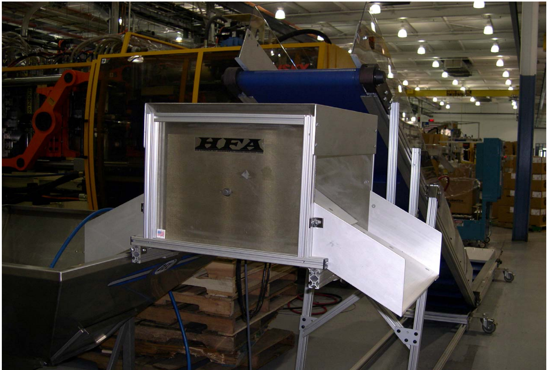
HFA 2230 Model Conveyor Feeding Diverter Along Side of Press
