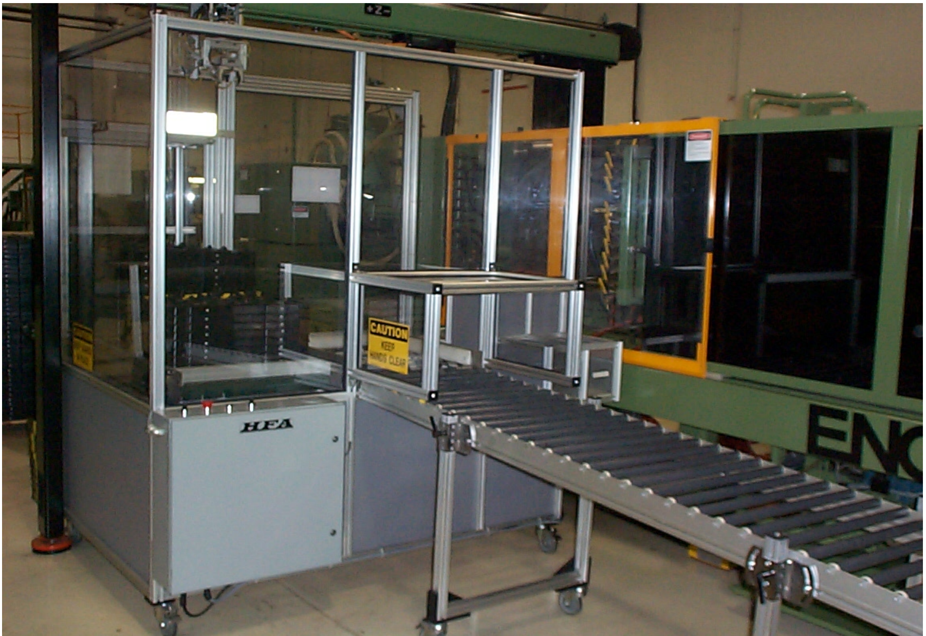
2270 Gravity roller off a Box-Fill System
