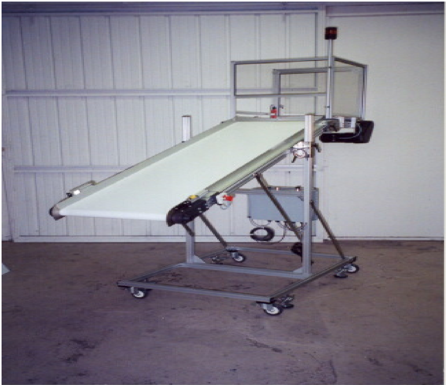
HFA 2240 Model Conveyor with White Textured Belt and Robot Guarding
