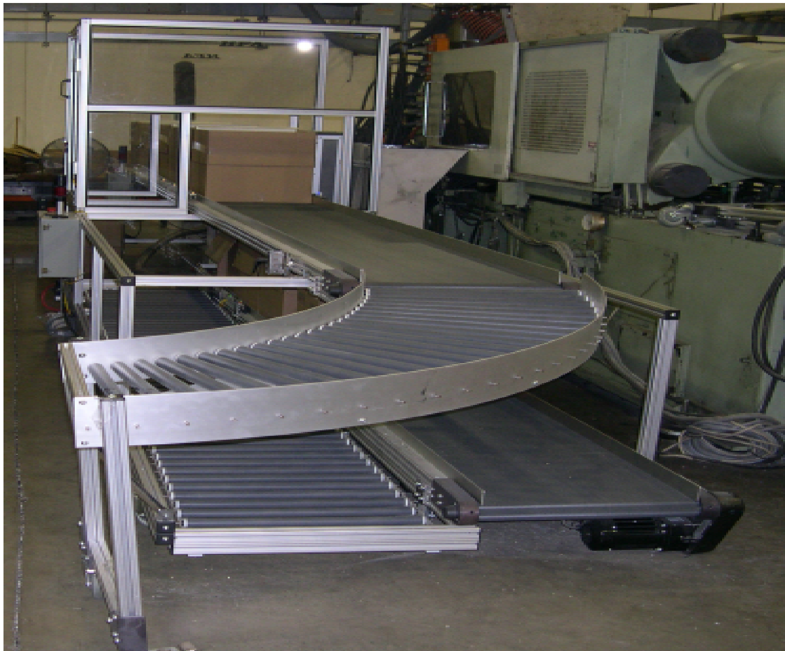
2270 Gravity roller with a 90° Curve
