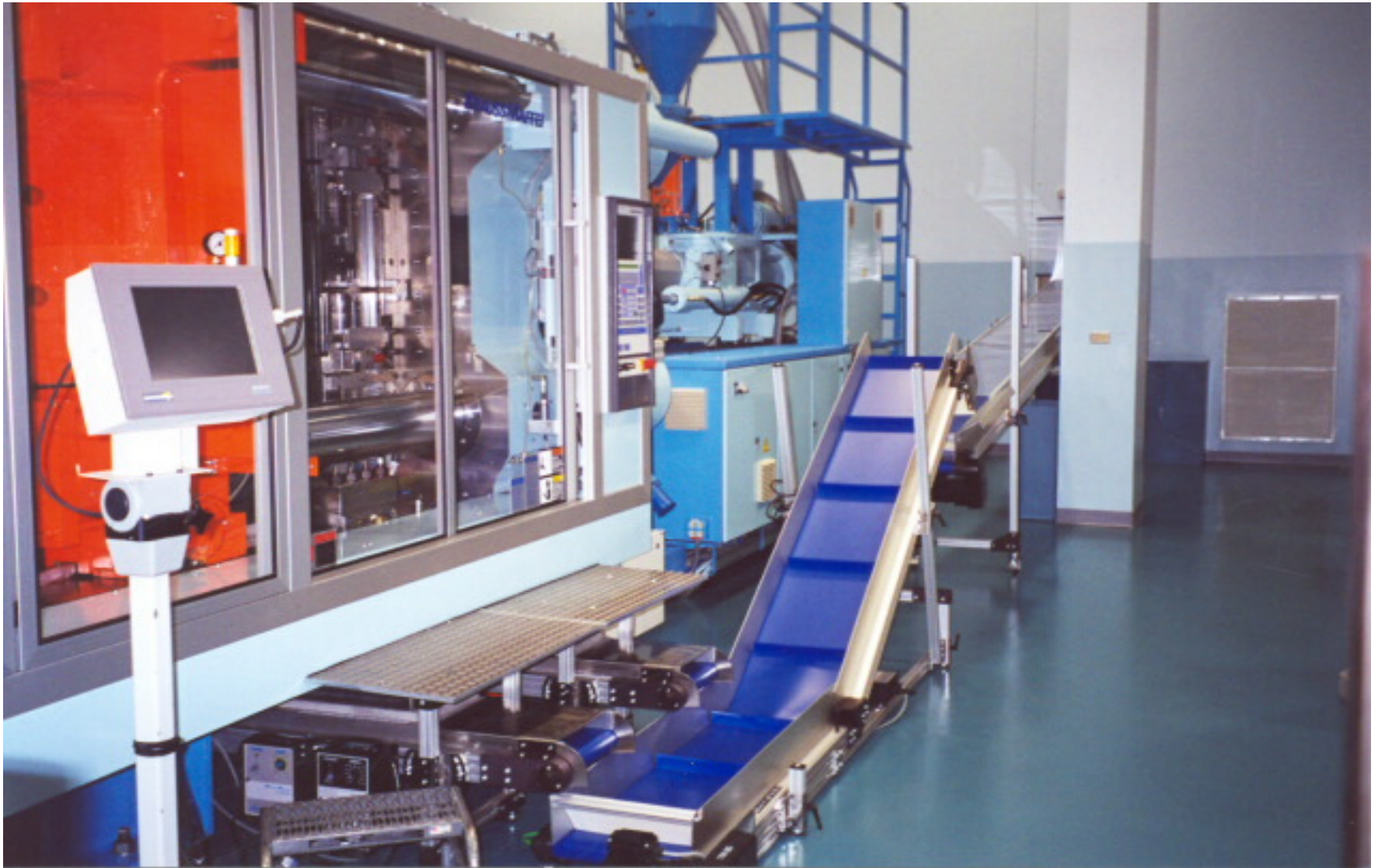
HFA 2210 Model Conveyors Feeding 2230's Going Thru the Wall Shown with Diamond-Plate Steps
