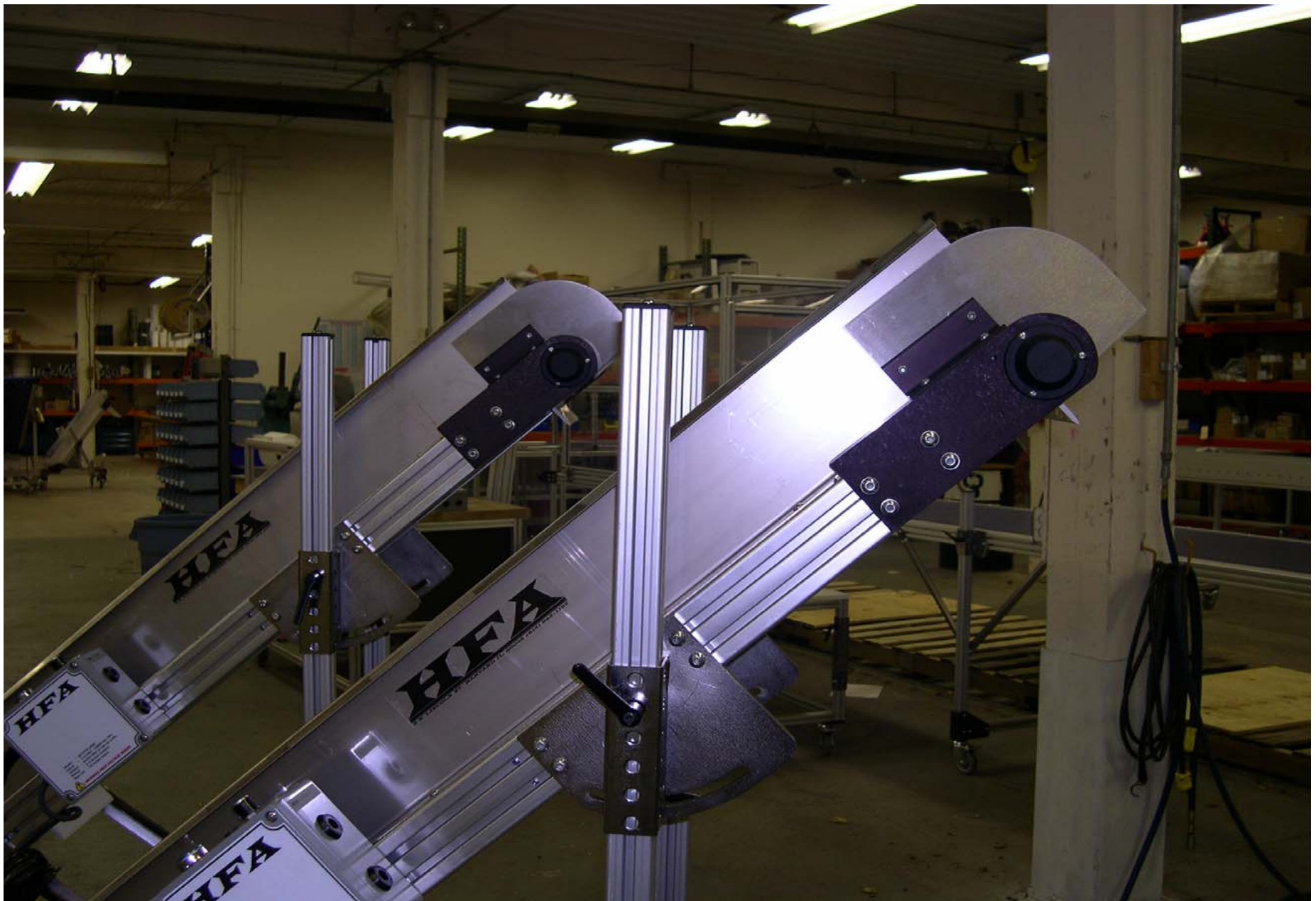
2220 with Stainless Steel Side Rails and Take-Up Rails
