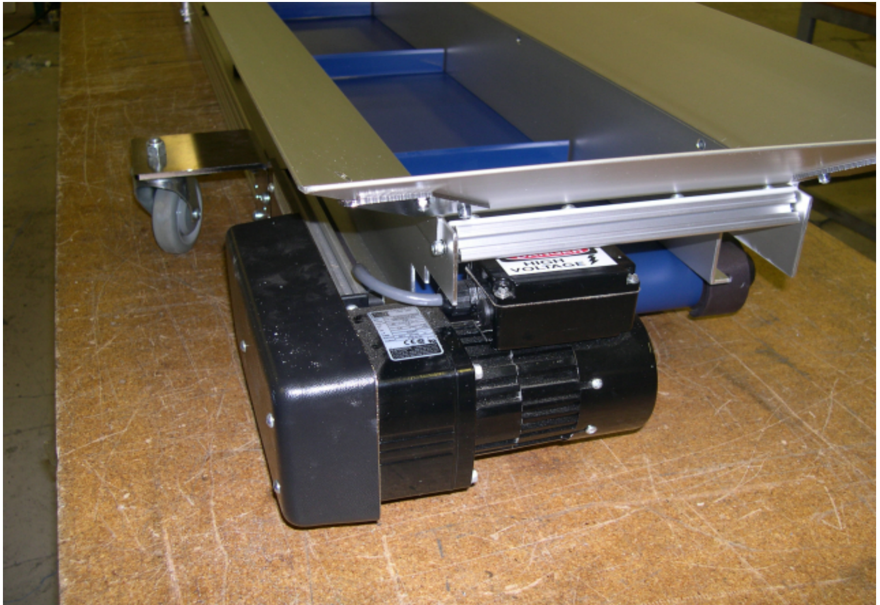
2230 with Flared Side Rails and Off-End Motor
