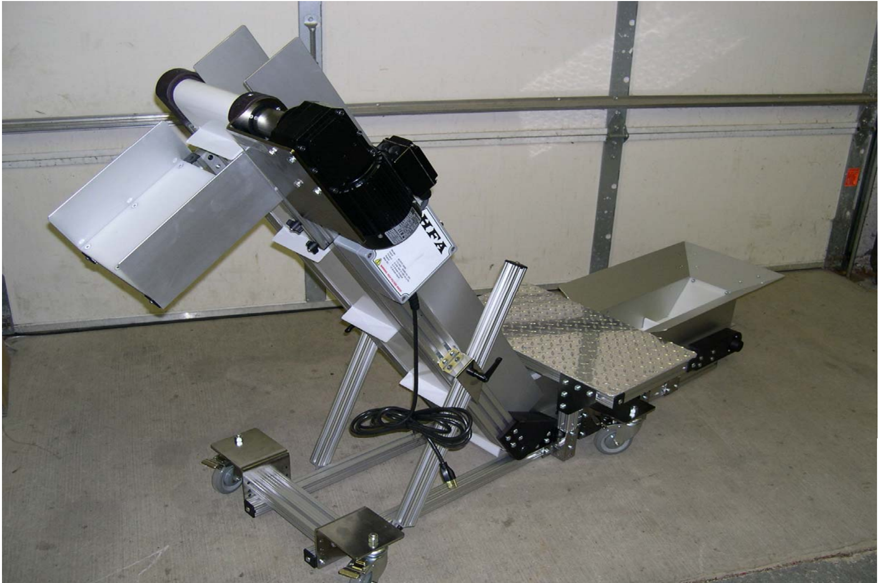
2230 with Step-Plate, Flared In feed Rails, Right-Angle Motor and Discharge Tray
