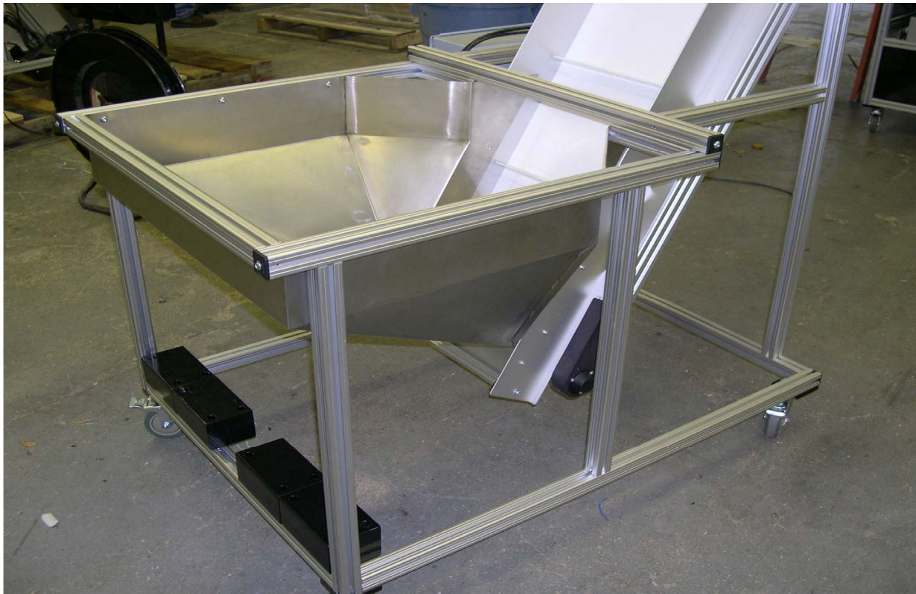
2260 Elevator with Custom-sized In-feed Hopper
