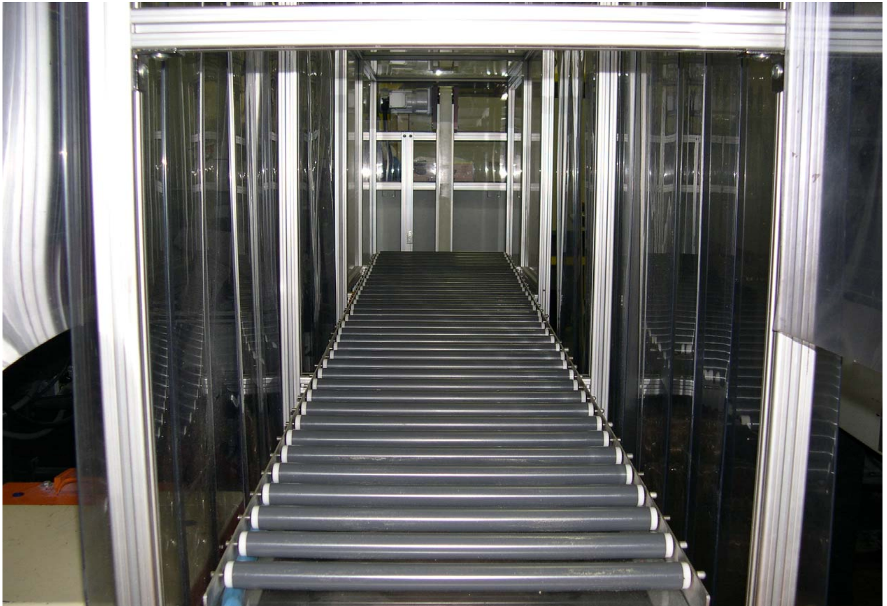
2270 Gravity Roller on Top-Level of Auto-Q2 Box-Fill System
