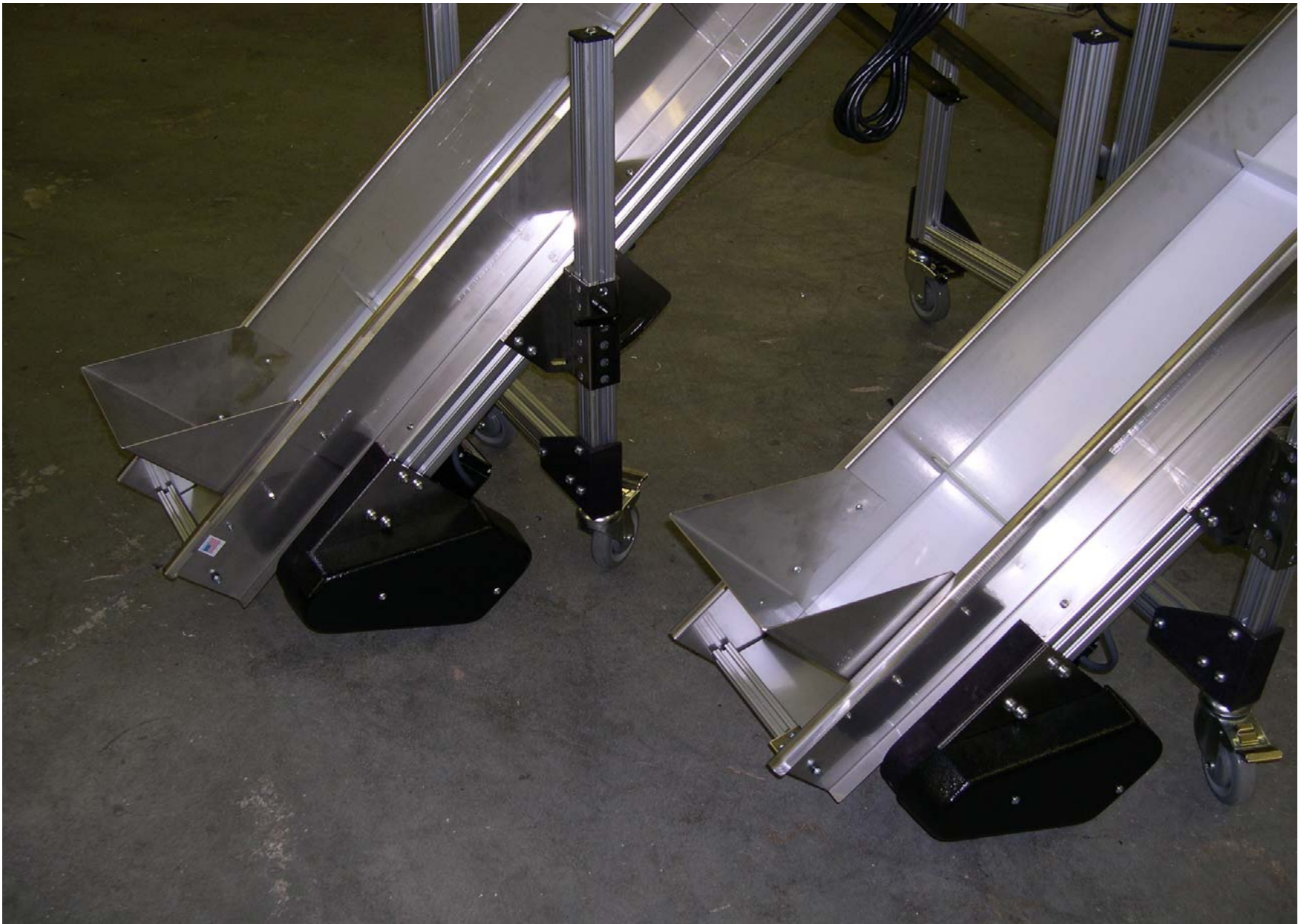
2220 with Stainless Rails and Standard In-feed Hopper
