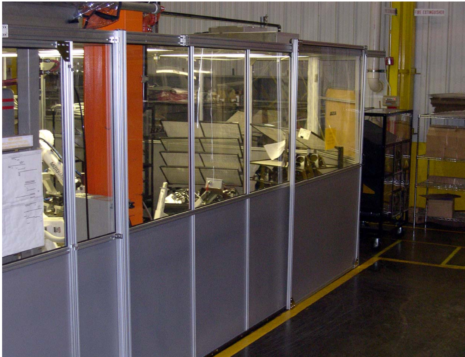
Stationary Clean-room Surrounding Presses and Robots
